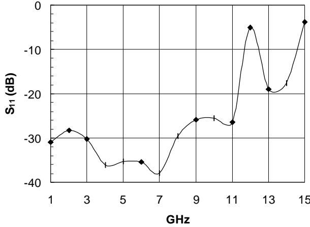
Fig. 2. S_{11} of the proposed transition, which consists of 5 sections each of length equals to 1 mm. S_{11} is less than -25 dB up to 11 GHz.
